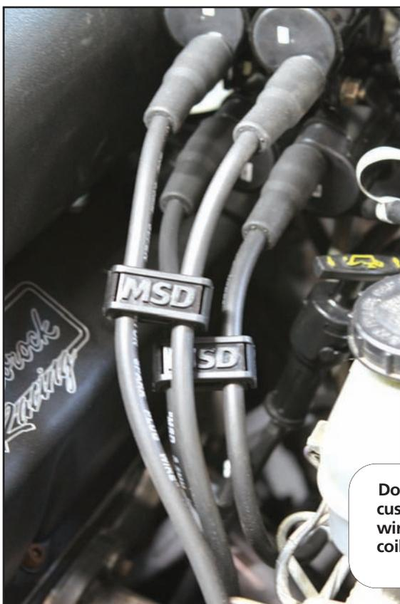
Doug Paradise of Dez Racing custom fit MSD 8.5mm spark plug wires from the firewall mounted coils to each spark plug.
