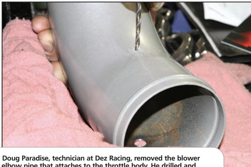
Doug Paradise, technician at Dez Racing, removed the blower elbow pipe that attaches to the throttle body. He drilled and tapped two holes on either side of it for the nozzle placement.
