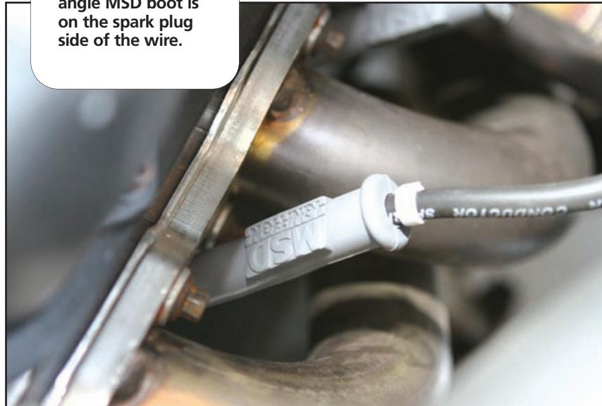
The standard multi-angle MSD boot is on the spark plug side of the wire.
