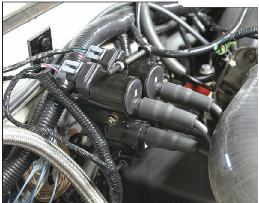
Pro-M Racing provides a billet cap to top off the distributor. The distributor acts as a crank and cam sensor for the ECU.
