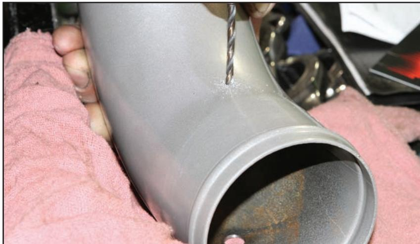
Doug Paradise, technician at Dez Racing, removed the blower elbow pipe that attaches to the throttle body. He drilled and tapped two holes on either side of it for the nozzle placement.
