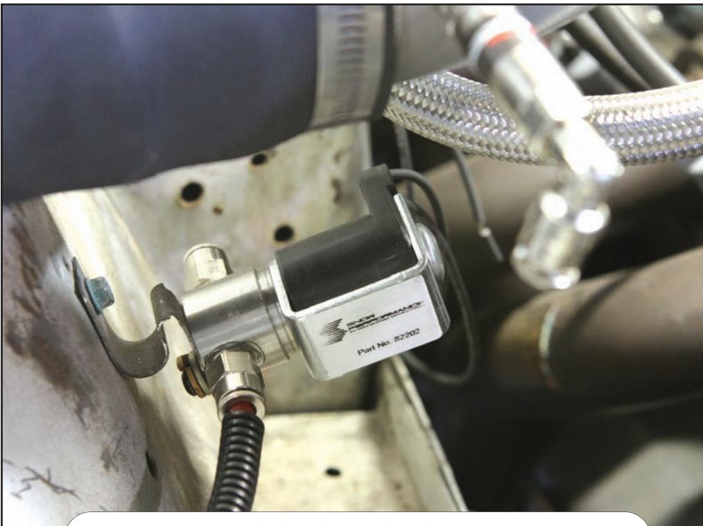
The Snow Performance solenoid acts in the same manner as a nitrous system solenoid. It controls the flow of water/meth into the engine. Snow Performance includes a special controller unit to activate the solenoid. The solenoid has a single feed that branches into two separate nozzles after the solenoid.
