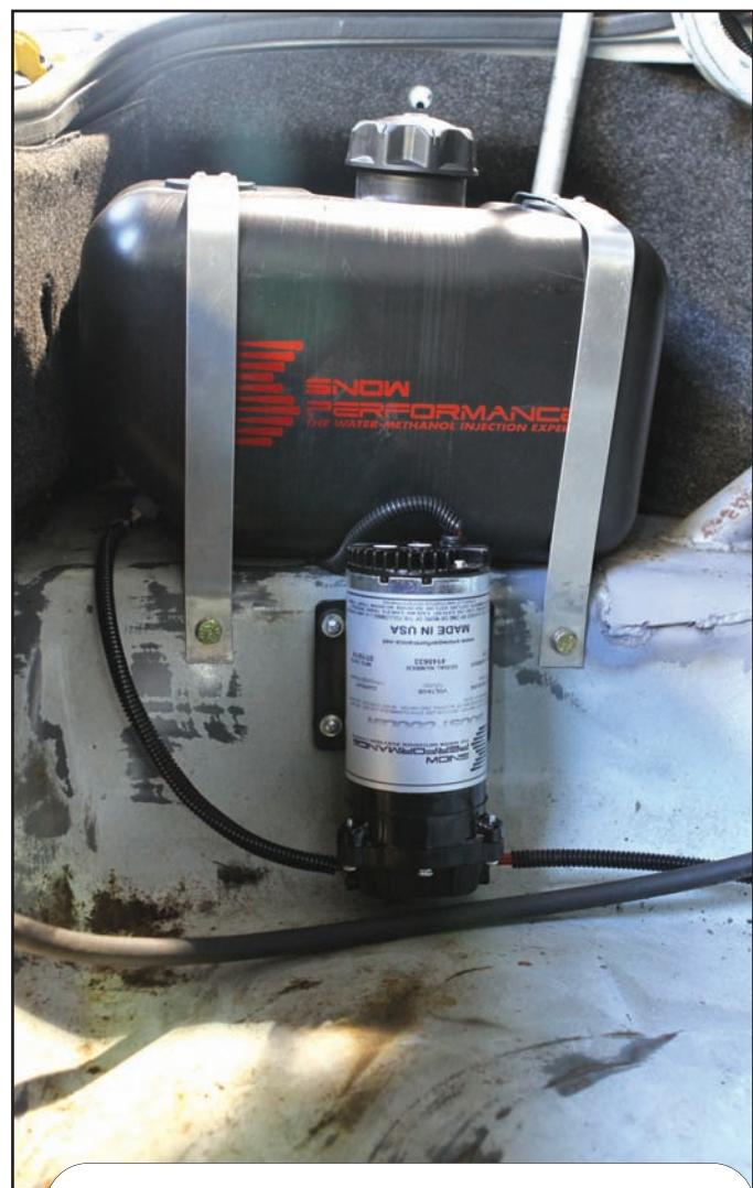
The large tank is placed in the trunk and the Snow Performance pump is mounted right next to it. Paradise and Dez Racing find this to be the easiest spot to mount the tank in Fox-body coupe cars. We aren't carrying a spare tire anyway so the pump bolts in nicely using the spare tire well.
